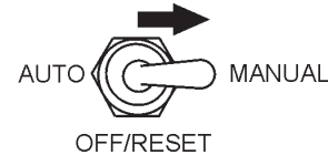
Figure 38. MPEC Control Switch (Manual Position)
